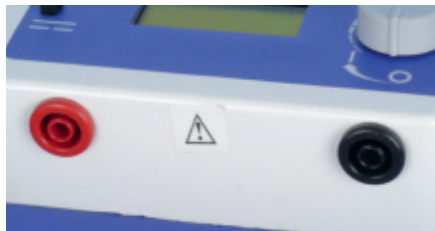
(3) Sockets to connect cables to electrodes
